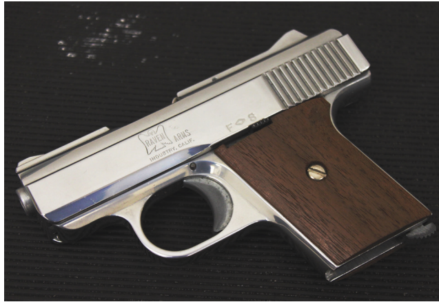
Figure 4.1 The Raven MP-25. Part of the identification markings are on left side of the slide (pictured); the model and caliber are on the opposite side. The serial number is stamped on the back strap of the grip. The Raven pistols are grouped as one of the Saturday night specials; untold millions were made, and they routinely turn up. (Image from author's collection.)
